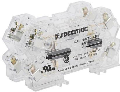
Socomec auxiliary contact, left or right side mount, (1) N.O./(1) N.C. contact(s), 6A @ 120 VAC/2.2A @ 120 VDC. Package of 2. For use with FUSERBLOC 30-200A switch bodies.
