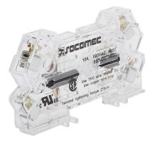
Socomec auxiliary contact, left or right side mount, (1) N.O./(1) N.C. contact(s), 6A @ 120 VAC/2.2A @ 120 VDC. For use with FUSERBLOC 30-200A switch bodies.
