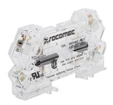
Socomec auxiliary contact, left or right side mount, (1) N.O./(1) N.C. contact(s), 6A @ 120 VAC/2.2A @ 120 VDC. For use with FUSERBLOC 30-200A switch bodies.
