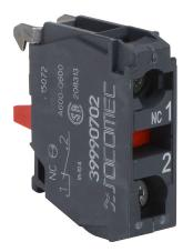
Socomec auxiliary contact, front mount, (1) N.C. contact(s), 6A @ 120 VAC/0.55A @ 120 VDC. For use with FUSERBLOC and FUSERBLOC Compact 30-600A Switch bodies.
