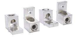
Socomec box type wiring lug, line or load mount, 1 openings, #4 AWG-600 MCM wire(s). Package of 4. For use with SIRCOVER 260-400A transfer switch bodies.
