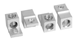
Socomec box type wiring lug, line or load mount, 1 openings, #6 AWG-300 MCM wire(s). Package of 4. For use with SIRCO and FUSERBLOC SERIES 200A switch bodies; SIRCOVER 100-200A transfer switch bodies.
