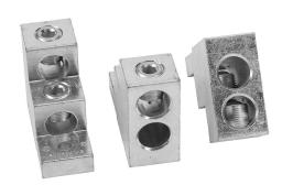
Socomec box type wiring lug, line or load mount, 2 openings, #2 AWG-600 MCM wire(s). Package of 3. For use with SIRCO and FUSERBLOC SERIES 600A switch bodies.
