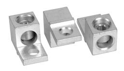
Socomec box type wiring lug, line or load mount, 1 openings, #6 AWG-300 MCM wire(s). Package of 3. For use with SIRCO and SIRCO DC 100-250A switch bodies.
