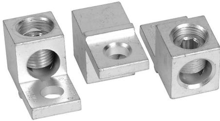
Socomec box type wiring lug, line or load mount, 1 openings, #6 AWG-300 MCM wire(s). Package of 3. For use with SIRCO and SIRCO DC 100-250A switch bodies.
