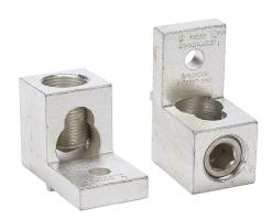
Socomec box type wiring lug, line or load mount, 1 openings, #4 AWG-600 MCM wire(s). Package of 2. For use with SIRCOVER 260-400A transfer switch bodies.
