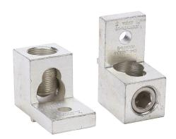
Socomec box type wiring lug, line or load mount, 1 openings, #4 AWG-600 MCM wire(s). Package of 2. For use with SIRCOVER 260-400A transfer switch bodies.
