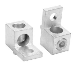
Socomec box type wiring lug, line or load mount, 1 openings, #6 AWG-300 MCM wire(s). Package of 2. For use with SIRCO and SIRCO DC 100-250A switch bodies.
