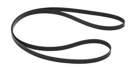
SureMotion timing belt, 0.08in MXL pitch, 1/4in wide, 390 tooth, 31.2in pitch length (circumference), polyurethane, polyester reinforced. Package of 3.
