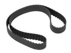
SureMotion timing belt, 3/8in L pitch, 1in wide, 104 tooth, 39in pitch length (circumference), neoprene, fiberglass reinforced.
