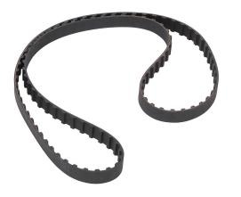
SureMotion timing belt, 3/8in L pitch, 1/2in wide, 104 tooth, 39in pitch length (circumference), neoprene, fiberglass reinforced.
