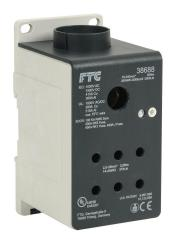
FTG enclosed power distribution block, finger-safe, 380A, 1-pole, line side: 1 opening accepts 500 kcmil to 2/0 AWG, load side: 6 openings accept 2 AWG to 14 AWG, panel or 35mm DIN rail mount, UL 1953 listed.
