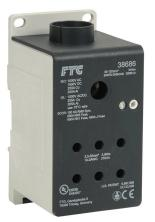
FTG enclosed power distribution block, finger-safe, 255A, 1-pole, line side: 1 opening accepts 250 kcmil to 2 AWG, load side: 6 openings accept 2 AWG to 14 AWG, panel or 35mm DIN rail mount, UL 1953 listed.
