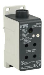
FTG enclosed power distribution block, finger-safe, 175A, 1-pole, line side: 1 opening accepts 2/0 AWG to 14 AWG, load side: 4 openings accept 2 AWG to 14 AWG, panel or 35mm DIN rail mount, UL 1953 listed.
