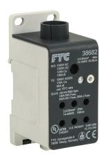
FTG enclosed power distribution block, finger-safe, 115A, 1-pole, line side: 1 opening accepts 1 AWG to 14 AWG, load side: 6 openings accept 4 AWG to 14 AWG, panel or 35mm DIN rail mount, UL 1953 listed.
