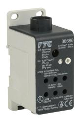
FTG enclosed power distribution block, finger-safe, 85A, 1-pole, line side: 1 opening accepts 3 AWG to 14 AWG, load side: 6 openings accept 8 AWG to 14 AWG, panel or 35mm DIN rail mount, UL 1953 listed.
