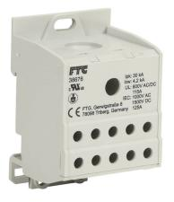
FTG enclosed terminal block, finger-safe, 115A, 1-pole, line side: 1 opening accepts 2 AWG to 8 AWG, load side: 10 openings accept 4 AWG to 14 AWG, panel or 35mm DIN rail mount, UL 1059 recognized.
