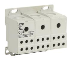
FTG enclosed terminal block, finger-safe, 115A, 3-pole, line side: 1 opening accepts 2 AWG to 8 AWG, load side: 6 openings accept 4 AWG to 14 AWG, panel or 35mm DIN rail mount, UL 1059 recognized.
