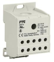
FTG enclosed terminal block, finger-safe, 175A, 1-pole, line side: 1 opening accepts 2/0 AWG to 8 AWG, load side: 10 openings accept 4 AWG to 14 AWG, panel or 35mm DIN rail mount, UL 1059 recognized.
