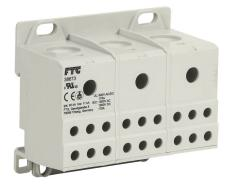
FTG enclosed terminal block, finger-safe, 175A, 3-pole, line side: 1 opening accepts 2/0 AWG to 8 AWG, load side: 6 openings accept 4 AWG to 14 AWG, panel or 35mm DIN rail mount, UL 1059 recognized.
