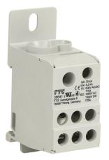
FTG enclosed terminal block, finger-safe, 115A, 1-pole, line side: 1 opening accepts 2 AWG to 8 AWG &1 opening accepts 4 AWG to 14 AWG, load side: 6 openings accept 4 AWG to 14 AWG, panel or 35mm DIN rail mount, UL 1059 recognized.
