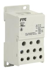
FTG enclosed terminal block, finger-safe, 225A, 1-pole, line side: 1 opening accepts 250 kcmil to 2 AWG, load side: 2 openings accept 2 AWG to 14 AWG & 5 openings accept 6 AWG to 14 AWG & 4 openings accept 8 AWG to 14 AWG, panel or 35mm DIN rail mount.
