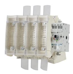
Socomec FUSERBLOC series rotary disconnect switch, fusible, Class J, load break capable, 4-pole, 600 VAC/250 VDC, 200A, 200kA SCCR, panel mount, UL 98 rated, front or side operated, accepts 10 x 10mm size shaft.
