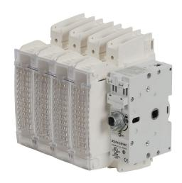
Socomec FUSERBLOC series rotary disconnect switch, fusible, Class J, load break capable, 4-pole, 600 VAC/250 VDC, 100A, 200kA SCCR, panel mount, UL 98 rated, front or side operated, accepts 10 x 10mm size shaft.
