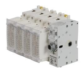
Socomec FUSERBLOC series rotary disconnect switch, fusible, Class J, load break capable, 4-pole, 600 VAC/250 VDC, 60A, 100kA SCCR, DIN rail or panel mount, UL 98 rated, front or side operated, accepts 10 x 10mm size shaft.
