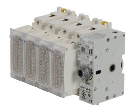
Socomec FUSERBLOC series rotary disconnect switch, fusible, Class J, load break capable, 4-pole, 600 VAC/250 VDC, 30A, 200kA SCCR, DIN rail or panel mount, UL 98 rated, front or side operated, accepts 10 x 10mm size shaft.
