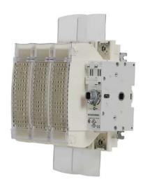
Socomec FUSERBLOC series rotary disconnect switch, fusible, Class J, load break capable, 3-pole, 600 VAC/250 VDC, 200A, 200kA SCCR, panel mount, UL 98 rated, front or side operated, accepts  $10 \times 10 \text{mm}$  size shaft.
