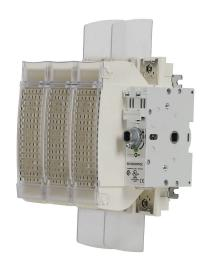
Socomec FUSERBLOC series rotary disconnect switch, fusible, Class J, load break capable, 3-pole, 600 VAC/250 VDC, 200A, 200kA SCCR, panel mount, UL 98 rated, front or side operated, accepts 10 x 10mm size shaft.
