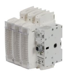
Socomec FUSERBLOC series rotary disconnect switch, fusible, Class J, load break capable, 3-pole, 600 VAC/250 VDC, 100A, 200kA SCCR, panel mount, UL 98 rated, front or side operated, accepts 10 x 10mm size shaft.
