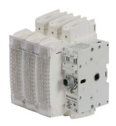
Socomec FUSERBLOC series rotary disconnect switch, fusible, Class J, load break capable, 3-pole, 600 VAC/250 VDC, 100A, 200kA SCCR, panel mount, UL 98 rated, front or side operated, accepts  $10 \times 10 \text{mm}$  size shaft.
