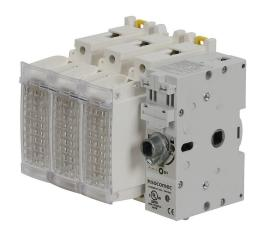
Socomec FUSERBLOC series rotary disconnect switch, fusible, Class J, load break capable, 3-pole, 600 VAC/250 VDC, 30A, 200kA SCCR, DIN rail or panel mount, UL 98 rated, front or side operated, accepts 10 x 10mm size shaft.
