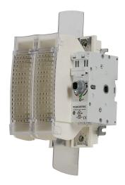
Socomec FUSERBLOC series rotary disconnect switch, fusible, Class J, load break capable, 2-pole, 600 VAC/250 VDC, 200A, 200kA SCCR, panel mount, UL 98 rated, front or side operated, accepts 10 x 10mm size shaft.
