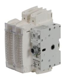
Socomec FUSERBLOC series rotary disconnect switch, fusible, Class J, load break capable, 2-pole, 600 VAC/250 VDC, 100A, 200kA SCCR, panel mount, UL 98 rated, front or side operated, accepts 10 x 10mm size shaft.
