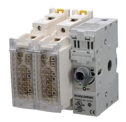
Socomec FUSERBLOC series rotary disconnect switch, fusible, Class J, load break capable, 2-pole, 600 VAC/250 VDC, 60A, 100kA SCCR, DIN rail or panel mount, UL 98 rated, front or side operated, accepts 10 x 10mm size shaft.
