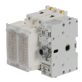
Socomec FUSERBLOC series rotary disconnect switch, fusible, Class J, load break capable, 2-pole, 600 VAC/250 VDC, 30A, 200kA SCCR, DIN rail or panel mount, UL 98 rated, front or side operated, accepts 10 x 10mm size shaft.
