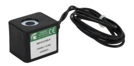
Spartan solenoid coil, 12 VDC, 6.5W, 18in 22AWG pigtail. For use with 3516 series Spartan valves.
