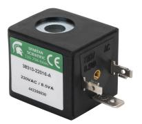
Spartan solenoid coil, 220 VAC, 8.5 VA, 18mm DIN style wiring plug. For use with 3516 series Spartan valves.
