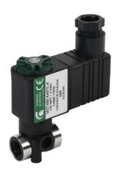
Spartan solenoid valve, 2-way, 2-position, N.C., glass-filled nylon body, 1/8in female NPT inlet(s), 1/8in female NPT outlet(s), Cv=0.31, 75 psi maximum operating pressure, 120 VAC operating voltage, 18mm DIN style wiring plug.
