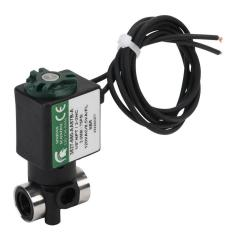
Spartan solenoid valve, 2-way, 2-position, N.C., glass-filled nylon body, 1/8in female NPT inlet(s), 1/8in female NPT outlet(s), Cv=0.31, 75 psi maximum operating pressure, 120 VAC operating voltage, 18in 22 AWG pigtail.
