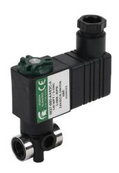
Spartan solenoid valve, 2-way, 2-position, N.C., glass-filled nylon body, 1/8in female NPT inlet(s), 1/8in female NPT outlet(s), Cv=0.31, 60 psi maximum operating pressure, 24 VDC operating voltage, 18mm DIN style wiring plug.
