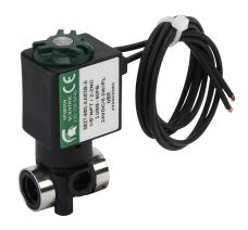
Spartan solenoid valve, 2-way, 2-position, N.C., glass-filled nylon body, 1/8in female NPT inlet(s), 1/8in female NPT outlet(s), Cv=0.31, 60 psi maximum operating pressure, 24 VDC operating voltage, 18in 22 AWG pigtail.
