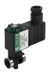
Spartan solenoid valve, 2-way, 2-position, N.C., glass-filled nylon body, 1/8in female NPT inlet(s), 1/8in female NPT outlet(s), Cv=0.24, 200 psi maximum operating pressure, 120 VAC operating voltage, 11mm DIN style wiring plug.
