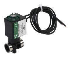
Spartan solenoid valve, 2-way, 2-position, N.C., glass-filled nylon body, 1/8in female NPT inlet(s), 1/8in female NPT outlet(s), Cv=0.24, 200 psi maximum operating pressure, 120 VAC operating voltage, 18in 22 AWG pigtail.
