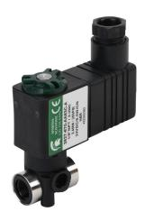
Spartan solenoid valve, 2-way, 2-position, N.C., glass-filled nylon body, 1/8in female NPT inlet(s), 1/8in female NPT outlet(s), Cv=0.24, 200 psi maximum operating pressure, 24 VDC operating voltage, 11mm DIN style wiring plug.
