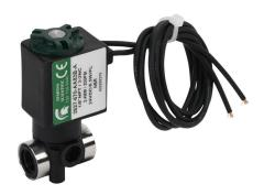
Spartan solenoid valve, 2-way, 2-position, N.C., glass-filled nylon body, 1/8in female NPT inlet(s), 1/8in female NPT outlet(s), Cv=0.24, 200 psi maximum operating pressure, 24 VDC operating voltage, 18in 22 AWG pigtail.
