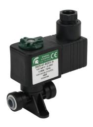
Spartan solenoid valve, 2-way, 2-position, N.C., acetal body, 1/4in push-to-connect tubing inlet(s), 1/4in push-to-connect tubing outlet(s), Cv=0.31, 75 psi maximum operating pressure, 120 VAC operating voltage, 18mm DIN style wiring plug.
