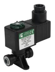
Spartan solenoid valve, 2-way, 2-position, N.C., acetal body, 1/4in push-to-connect tubing inlet(s), 1/4in push-to-connect tubing outlet(s), Cv=0.31, 60 psi maximum operating pressure, 24 VDC operating voltage, 18mm DIN style wiring plug.
