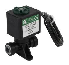
Spartan solenoid valve, 2-way, 2-position, N.C., acetal body, 1/4in push-to-connect tubing inlet(s), 1/4in push-to-connect tubing outlet(s), Cv=0.31, 75 psi maximum operating pressure, 120 VAC operating voltage, 18in 22 AWG pigtail.
