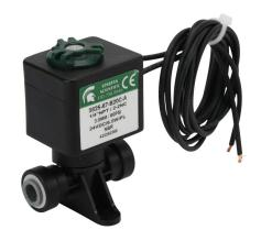
Spartan solenoid valve, 2-way, 2-position, N.C., acetal body, 1/4in push-to-connect tubing inlet(s), 1/4in push-to-connect tubing outlet(s), Cv=0.31, 60 psi maximum operating pressure, 24 VDC operating voltage, 18in 22 AWG pigtail.
