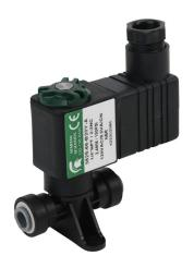
Spartan solenoid valve, 2-way, 2-position, N.C., acetal body, 1/4in push-to-connect tubing inlet(s), 1/4in push-to-connect tubing outlet(s), Cv=0.24, 150 psi maximum operating pressure, 120 VAC operating voltage, 11mm DIN style wiring plug.
