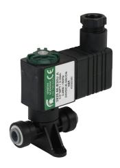
Spartan solenoid valve, 2-way, 2-position, N.C., acetal body, 1/4in push-to-connect tubing inlet(s), 1/4in push-to-connect tubing outlet(s), Cv=0.24, 150 psi maximum operating pressure, 24 VDC operating voltage, 11mm DIN style wiring plug.
